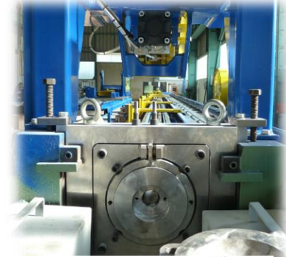
High power drawing machine
