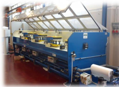
Multistep drawing machine
