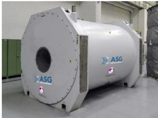
11.7 T 68 cm MRI Passively Shielded Head Scanner to be commissioned, NIH Clinical Center, Bethesda, USA – Gachon Medical University, Seoul, Korea
