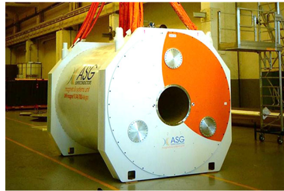
11.7 T 68 cm MRI Passively Shielded Head Scanner to be commissioned, NIH Clinical Center, Bethesda, USA – Gachon Medical University, Seoul, Korea
