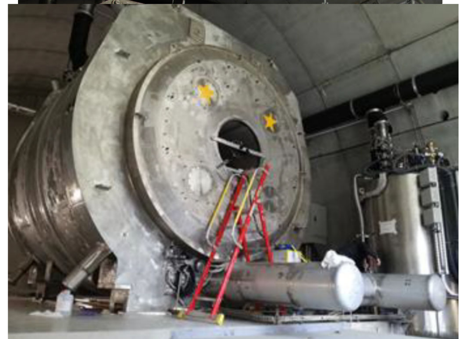
Final leak tests (inner cooling circuits and vacuum vessel) Leak rate of 5 \cdot 10^{-9} mbar.l/s on all the internal cooling circuits
