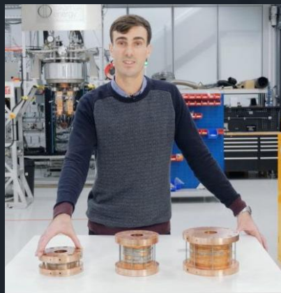
Franken Coil Stack of QA coils (2018) 15 T peak field on coil
