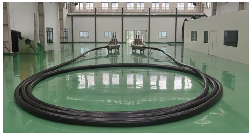
100m, \pm 375\text{V}/4500\text{ A} DC Superconducting Cable
