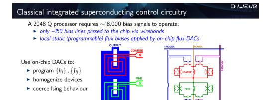
X/Y/Z addressing scheme uses ~82 wires to address ~36,000 DAC "loops" ~22 kilobytes of on-chip memory ~1 megabyte/s
