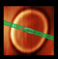
Dissipation dominated by edge defects in graphene
