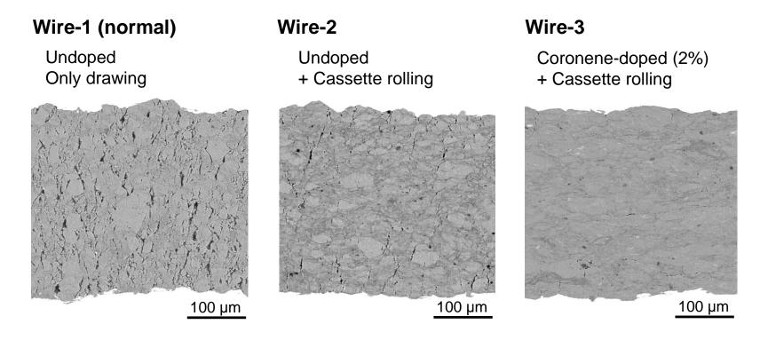
Coronene addition and cassette rolling are effective to obtain a well-connected core.
