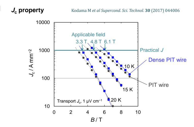
The dense PIT wire has higher applicable fields than the PIT wire.
