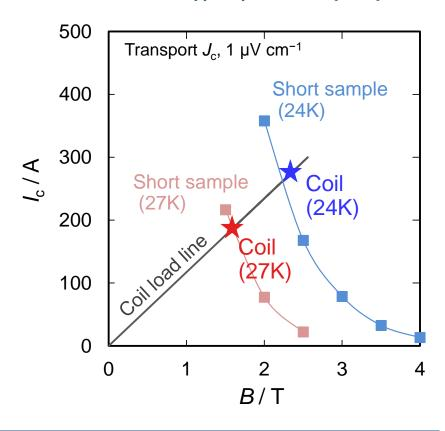
The coil was successfully driven in I = 286 A and  $B_{\text{max}} = 2.3$  T at 24 K. The coil  $I_{\text{c}}$  is nearly equal to the value expected from the short sample.
