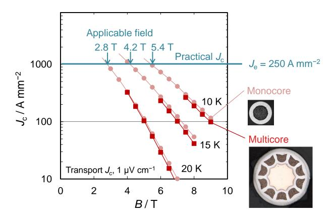
The  $J_{\rm c}$  of multicore wire is almost the same as that of monocore wire.
