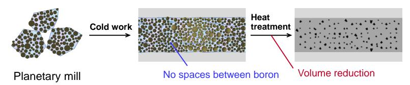
Partial generation of MgB<sub>2</sub> (Mechanical alloying)
