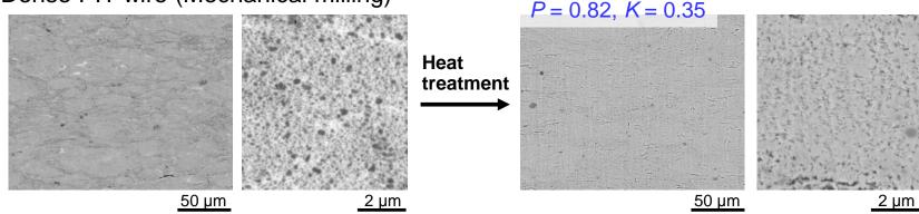
We confirmed higher packing factor and higher connectivity for the dense PIT wire.
