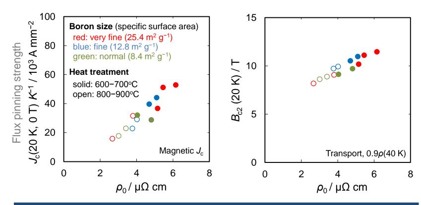
The use of finer boron powder and lower-temperature heat-treatment make  $MgB_2$  dirtier, resulting in the improvement of flux pinning strength and  $B_{c2}$ .
