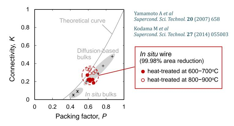
The cold work with the large area reduction is essential to enhance the packing factor and connectivity.
