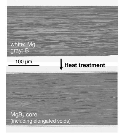
The size of MgB<sub>2</sub> cores is homogeneous and MgB<sub>2</sub> is well connected.
