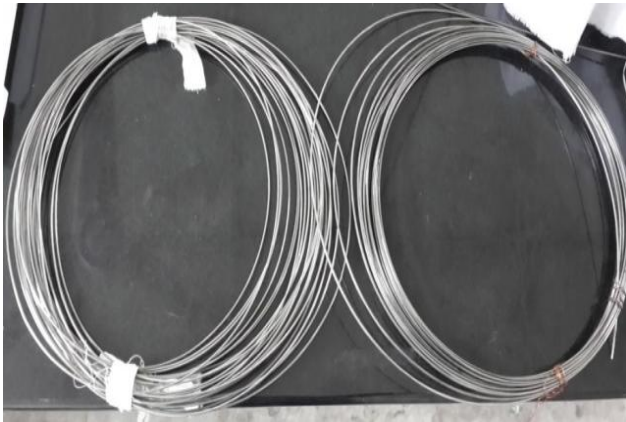
17 Mtrs long Mono filament & 6-filament strand with 2.29 mm O.D.
