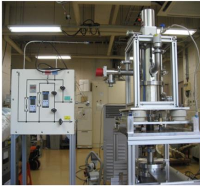
Developed closed cycle TS (Right) and gas flow control box (Left).
