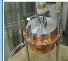
Evaporator in the center of rotor.
