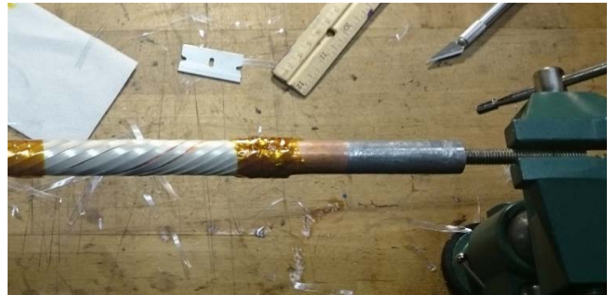
Cable after wrapping HTS tapes onto former
