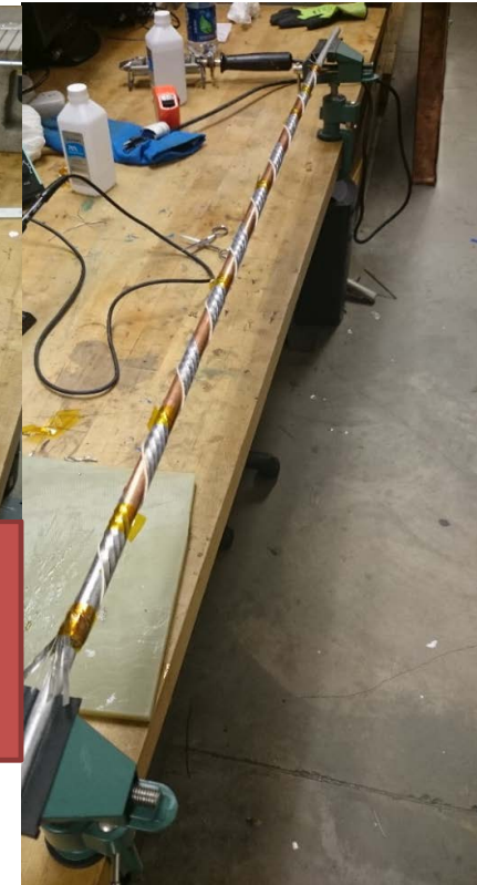
Heat Shrink Insulated HTS tape being wrapped onto former
