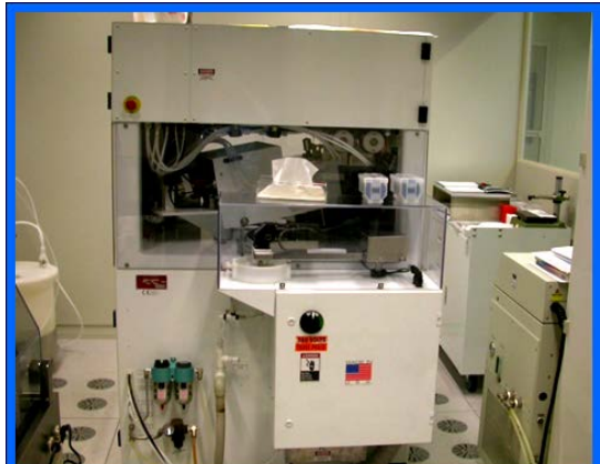
chem.- mechan. Polishing (CMP) planar layer interconnection
